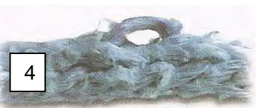
> Image 4 Strand reduced by 25% abrasion
