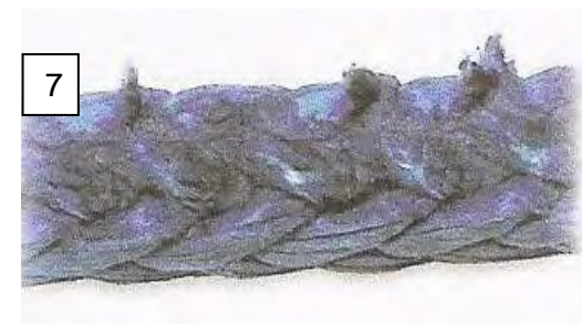
> Image 7 This rope has been exposed to extreme heat.
